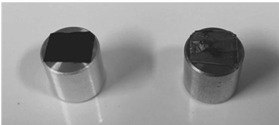
Fig 5. Changes in the Specimen Before (Left) and After (Right) Coating in the Ion Sputter Coater. Comparing before and after the coating process, it is observed that not only the surface of the specimen but also the stage has turned grey after coating, indicating that the entire specimen, along with its stage, has been uniformly coated.
