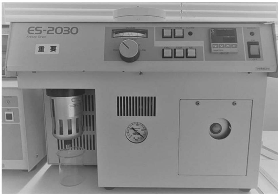
Fig 3. Freeze Vacuum Dryer (Hitachi ES-2030). The water contained in the hydrated sample for SEM would be dehydrated with ethyl alcohol, and substituted with t-butyl alcohol, and frozen in a freezer of  $-20^{\circ}\text{C}$  and then dried with sublimation at about 13.3 Pa in the evacuator of reduced pressure.
