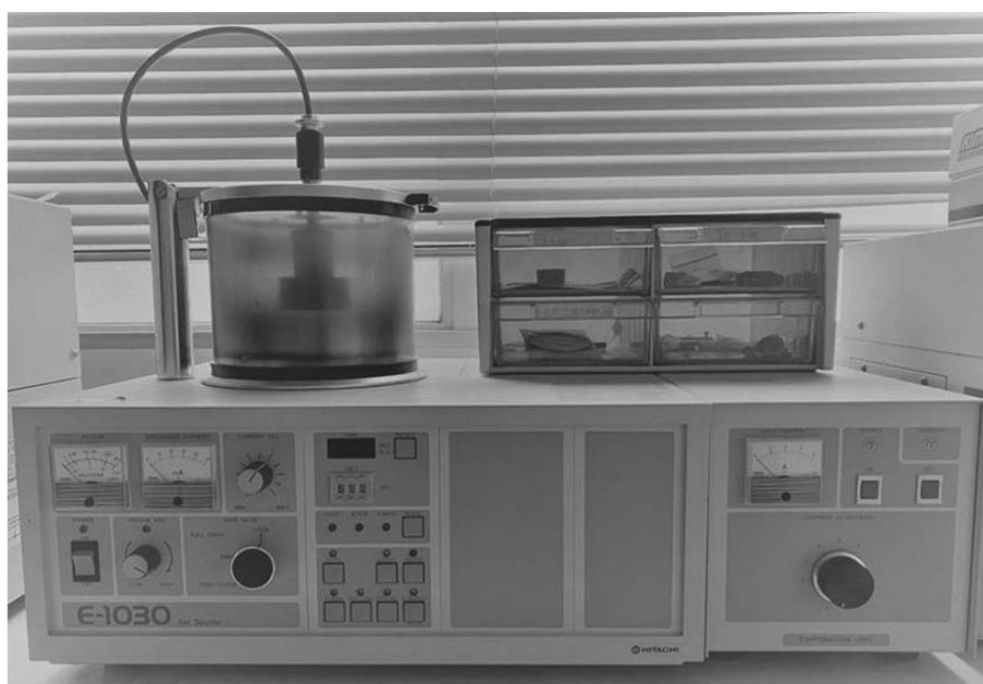
Fig 4. Ion Sputter Coater Hitachi E-1030. It is utilized in the preparation of non-conductive specimens for electron microscopy by applying a thin conductive coating on their surfaces. This process enhances the electrical conductivity of the specimens, preventing charging artifacts during microscopic observations and ensuring the acquisition of high-quality images and data.
