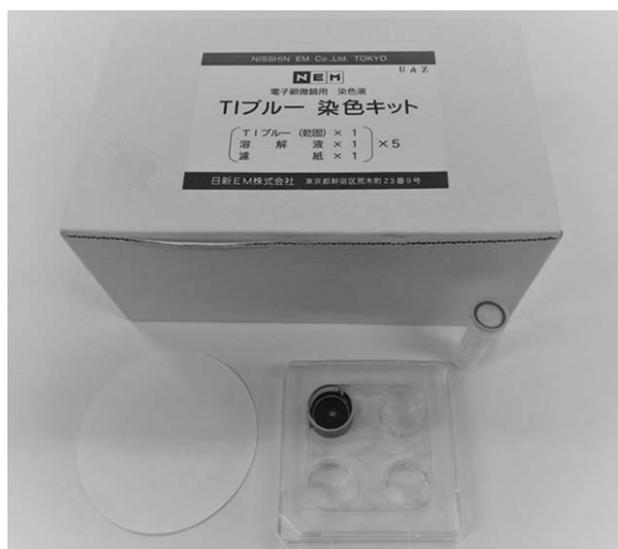
Fig 6. Platinum Blue (TI-Blue) Staining Kit. Previously, a significant drawback was that users had to personally prepare the platinum blue, and the synthesis reaction took about one week to complete. However, since its commercialization in 2008 by Nissin EM Co., Ltd. (as TI Blue), it has become readily available, allowing for easy use by anyone in the present day.
